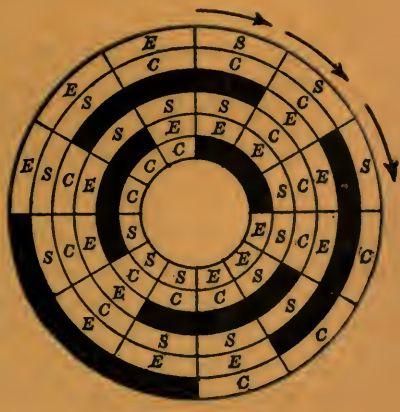
Three Cylinder Cranks-120° Fired 1-3-2
